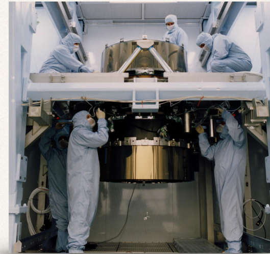
Assembly of Mirror shells (NASA/GSFC)
