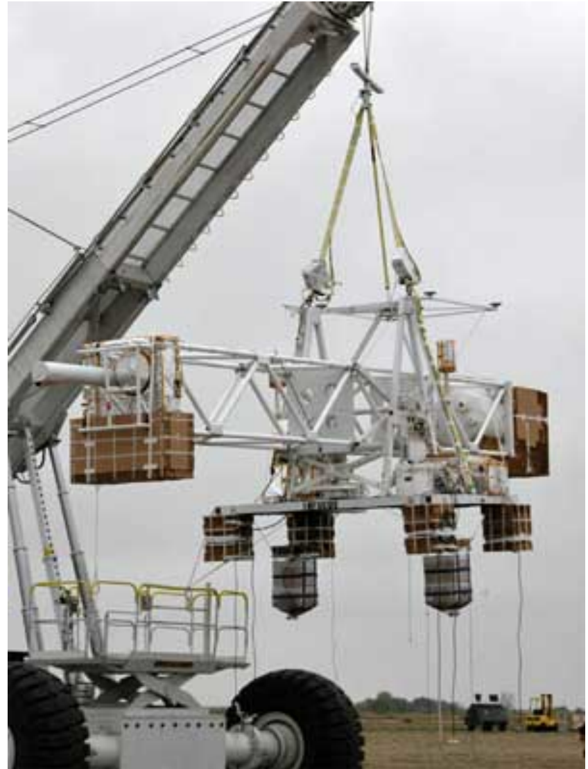
InFOCUS gondola with 8m optical bench (Tueller et al., NASA GSFC)
