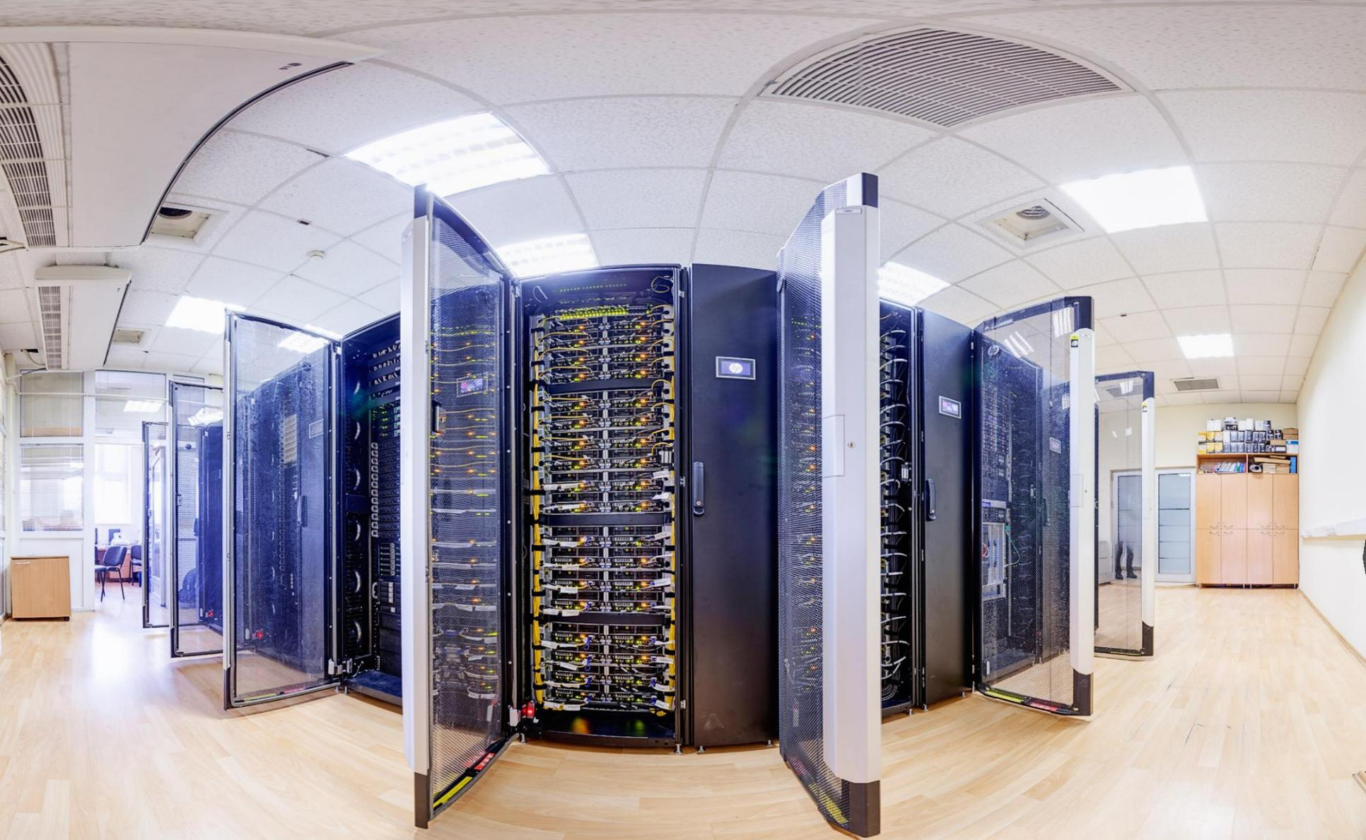
PARADOX Cluster at the Scientific Computing Laboratory of Institute of Physics Belgrade: 106 compute nodes (2 x 8 core Sandy Bridge Xeon 2.6GHz processors with 32GB of RAM + NVIDIA® Tesla™ M2090)
