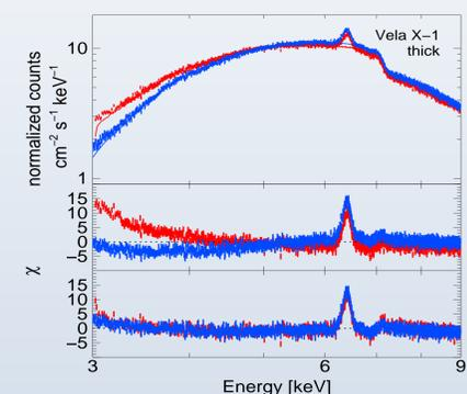
**Figure 6:** *Top:* Measured EPIC-pn Timing mode spectrum (blue) and Modified Timing mode spectrum generated from these data (red), fitted with an absorbed power-law. *Middle:* The redistribution of events in the Modified Timing mode leads to an apparent soft excess. *Bottom:* New response matrix for the Modified Timing mode fully describes the calibration of this mode (Fritz 2008).
