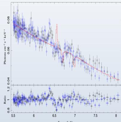
**Figure 5:** The best fit model (shown in red) to the same EPIC-pn data now compared to *Chandra* data (blue) shows clear disagreement in the position of 6.4 keV narrow emission line and resonant iron absorption lines (*Chandra* values by Hanke et al. 2009). Only when applying a gainshift of  $\sim 2\%$  to EPIC-pn data (as in the Fig. 3), agreement is reached.
