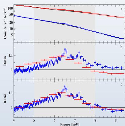
**Figure 4:** The effect of the gainshift correction, when applied on EPIC-pn data here fitted simultaneously with PCA data. Panel **b** represents the fit without the correction and with clear disagreement of the data, while panel **c** shows the improvement when corrected for gainshift of  $\sim 2\%$  (see **poster B05** for more details on the spectral analysis of these datasets of Cygnus X-1).
